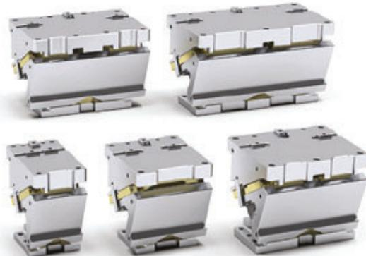
**GB** **CHW** cam units are extremely compact and suitable for applications requiring high work forces. They are equipped with sintered steel sliding elements (SINT300®) and thanks to the new stop system, the cam slider can be easily disassembled for quick maintenance. Four models with **working angles from 0° to 75°** (in 5° steps), **work forces from 210 to 320 kN**. **Working widths from 65 to 110 mm**.
