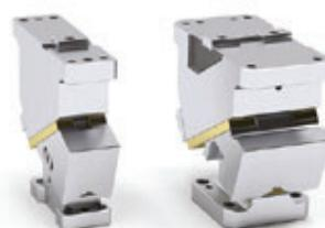
**GB** CLF aerial cam units are suited to make medium-light drilling and flanging workings. Two models with **work angles from 0° to 70°** (5° steps), **work forces from 116 to 192 kN**. **Slider widths from 80 to 150 mm**. Extraction only by enhanced coil spring.
