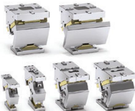
**(GB)** **CHR** aerial cam units are best suited for heavy drilling and flanging. **Six models** are available with **work angles from 0° to 60°** (in 5° steps), **work forces from 90 to 521 kN**. **Slider widths from 70 to 400 mm**. Manufactured according to **NAAMS** standards, these cam units are equipped with cam accelerators to quieten the noise level starting from 165 mm width. It is possible to choose between coil spring or gas spring return.
