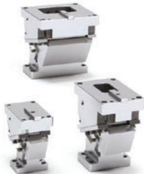
**(GB)** **CHK** aerial cam units are best suited for medium/light drilling and flanging. They look different from CLK due to the presence of a V guide on the Driver to improve alignment precision. **Three models** are available with **work angles from 0° to 70°** (in 5° steps for 65 mm width and 10° steps for 100 and 200 mm widths), **work forces from 58 to 231 kN**. **Slider widths from 65 to 200 mm**. Coil spring return only.
