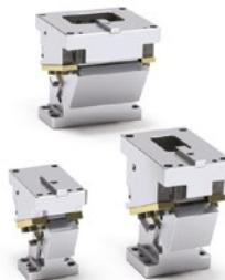
**④** **CHK** aerial cam units are best suited for medium/light drilling and flanging. They look different from CLK due to the presence of a V guide on the Driver to improve alignment precision. **Three models** are available with **work angles from 0° to 70°** (in 5° steps for 65 mm width and 10° steps for 100 and 200 mm widths), **work forces from 58 to 231 kN**. **Slider widths from 65 to 200 mm**. Coil spring return only.
