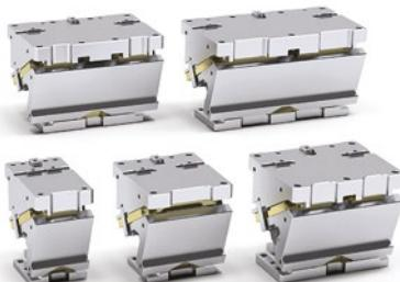
④ Our **CLB** cam units offer a very competitive performance /price ratio. Five models are available with **work angles from 0° to 60°** (in 5° steps), **work forces from 302 to 865 kN**, **slider widths from 200 to 600 mm**. It is possible to choose between **coil spring or gas spring return**.
