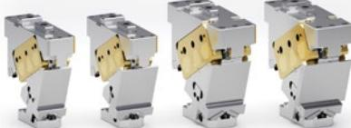
④ **CHW** cam units are extremely compact and suitable for applications requiring high work forces. They are equipped with sintered steel sliding elements (SINT300®) and thanks to the new stop system, the cam slider can be easily disassembled for quick maintenance. Four models with **working angles from 0° to 75°** (in 5° steps), **work forces from 210 to 320 kN**. **Working widths from 65 to 110 mm**.
