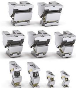
**GB** We recommend the **CHD** range of cam units for heavy-duty applications. Nine models are available with work angles from 0° to 65° (in 5° steps), work forces from 60 to 645 kN, slider widths from 50 to 300 mm. It is possible to choose between coil spring or gas spring return.
