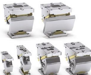
**④** **CHR** aerial cam units are best suited for heavy drilling and flanging. **Six models** are available with **work angles from 0° to 60°** (in 5° steps), **work forces from 90 to 521 kN**. **Slider widths from 70 to 400 mm**. Manufactured according to **NAAMS** standards, these cam units are equipped with cam accelerators to quieten the noise level starting from 165 mm width. It is possible to choose between coil spring or gas spring return.
