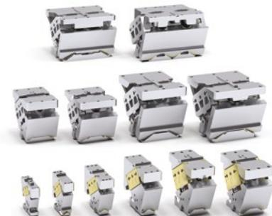
**GB** They are compact, have high work and return forces, are built from high-strength materials which ensure excellent resistance to twisting loads and have very good penetrating precision. They are characterized by easy maintenance thanks to the use of normalized wear plates (VDI3357) and to the possibility to change the gas spring under press. Twelve models are available with work angles from 0° to 75° (in 5° steps), work forces from 92 to 1202 kN, slider widths from 50 to 600 mm.
