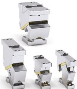
**(GB)** CLC aerial cam units are best suited for medium/light drilling and flanging. **Four models** are available with **work angles from 0° to 70°** (in 5° steps), **work forces from 41 to 140 kN**. **Slider widths from 50 to 150 mm**. Coil spring return only.
